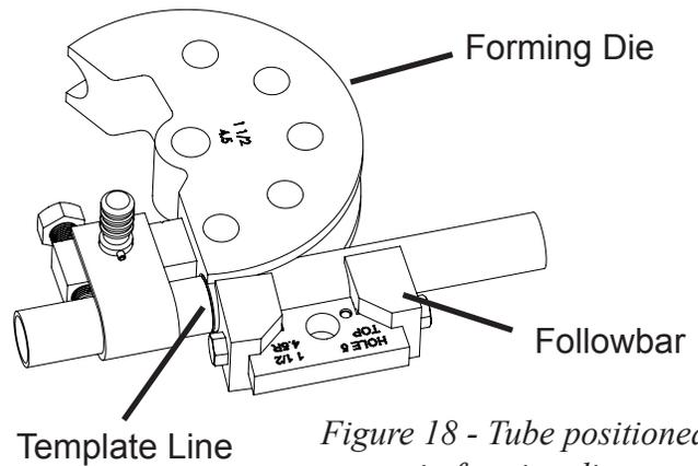
Figure 18 - Tube positioned in forming die
