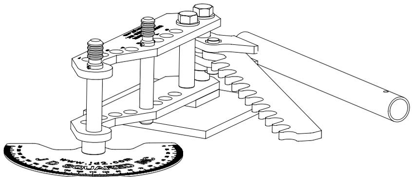
Figure 2 - Completed Frame Assembly with Degree Plate
