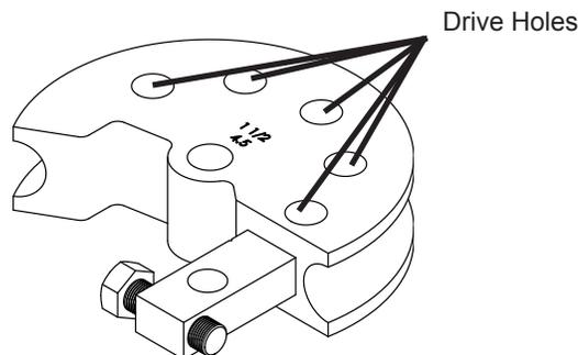
Figure 7 - Forming Die with drive holes
