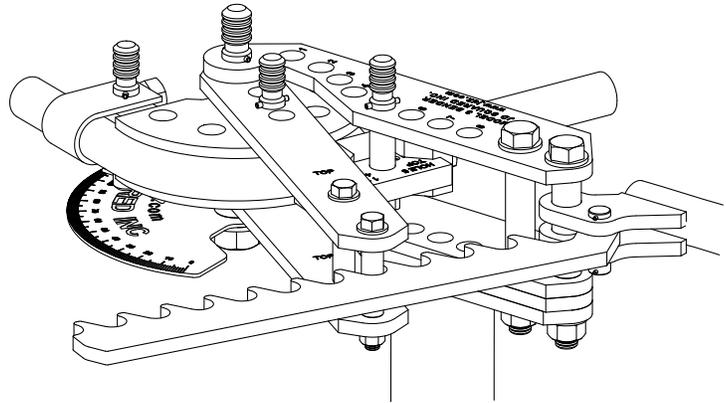
Figure 13 - Bending with drive holes and ratchet
