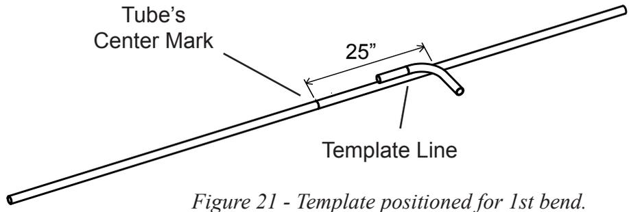
Figure 21 - Template positioned for 1st bend.
