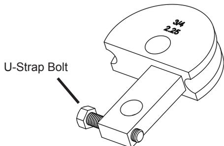
Figure 6 - Forming Die without drive holes
